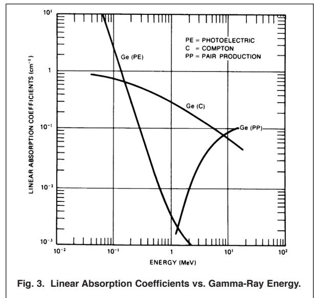
Fig. 3. Linear Absorption Coefficients vs. Gamma-Ray Energy.
