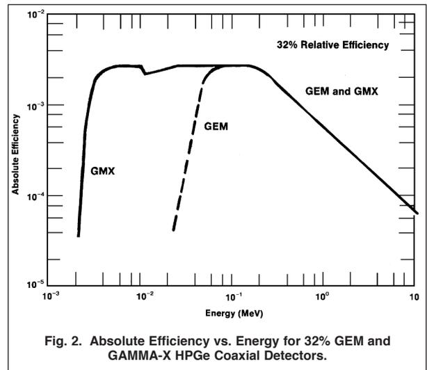
Fig. 2. Absolute Efficiency vs. Energy for 32% GEM and GAMMA-X HPGe Coaxial Detectors.
