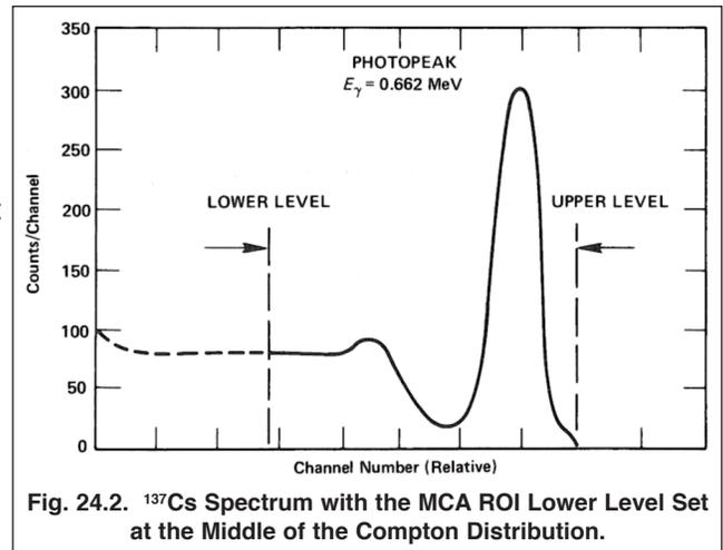
**Fig. 24.2.**  $^{137}\text{Cs}$  Spectrum with the MCA ROI Lower Level Set at the Middle of the Compton Distribution.
